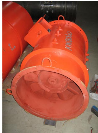
Figure 4: New axial ventilation fan
