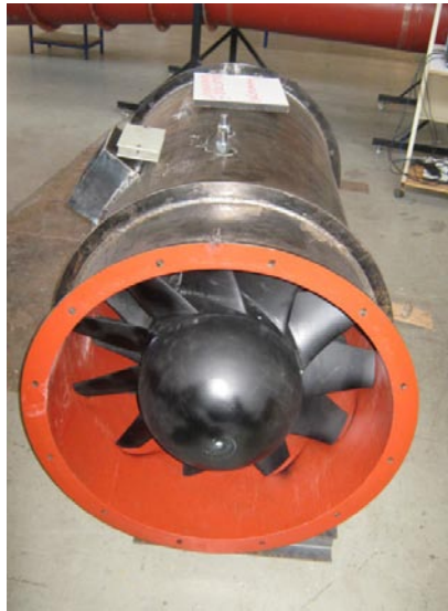
Figure 5: Existing steel axial ventilation fan
